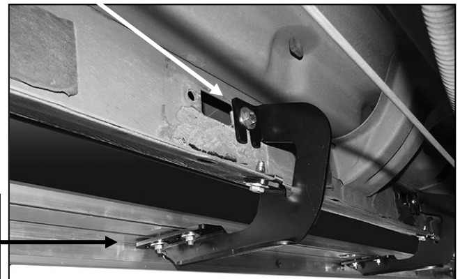
(Fig 9) Driver/left rear Bracket installed
