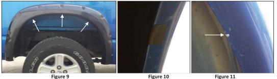
Remove white backing from black tabs and place half of the tab over the grease pencil mark and fold the other half over the 8. fender lip Figure 11.
