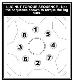
metal-to-metal contact at the wheel mounting surfaces can cause the lug nuts to loosen and the wheel to come off while the vehicle is in motion.
