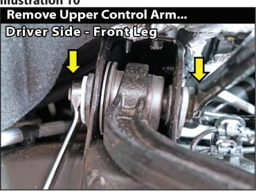
**MARNING:** Note that the new UCAs Must Be Greased BEFORE vehicle is Driven.
