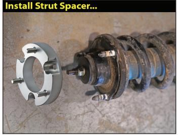
Install Lower Strut Mount... Driver Side
