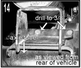
head sides) and Nyloc nut to attach the factory brake line bracket - to - Superlift bracket. Tighten the 7/16" hardware (50). Tighten the 5/16" hardware (200 in. Lbs.). Tighten the factory hardware (top hole) (23).
