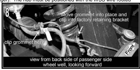
WSS wire and rubber grommet with a detergent-based cleaner (ex: Windex, Formula 409), which allows the WSS wire to slide easily through the rubber grommet. When satisfied with routing, insert the WSS wire / rubber grommet into the mounting bracket.
