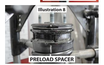
24. Once the strut spacer is securely fastened make sure the top of the factory studs do not extend past the top of the strut spacer, if they do they must be ground down below the spacer top plate for proper fitment in the vehicle.
