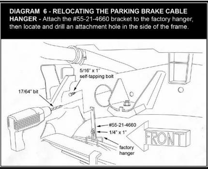
with the supplied 5/16" x 1" self-tapping bolt (13), then tighten the 1/4" bolt (76 in-lb.).
