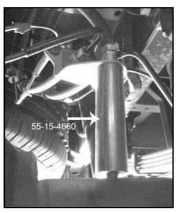
□ Reinsert the factroy bolt that retains the brake line to the rear of the spring perch. (35)
