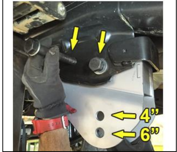
DIAGRAM 2C - RADIUS ARM DROP BRACKETS - Driver side shown.
