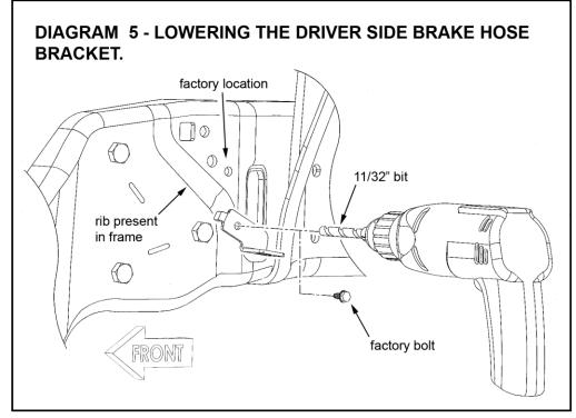
☐ Carefully push the bracket aside and drill at the marked location using an 11/32" bit. Put the bracket back into position and secure it using the factory self-tapping bolt in the drilled hole. Tighten to factory specifications.
