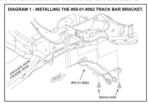
□ [DIAGRAM 1] Position the Superlift® track bar bracket (#55-01-9062) on the frame in the same place as the original and secure using the factory hardware. There are a total of five bolts; three attached to a retaining tab plus two additional bolts. Once all the bolts are started, tighten (136).
