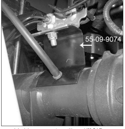
shocks using the factory hardware. On some models, it is necessary to position a 1/2" SAE washer (supplied) on either side of the lower shock bushing and its mount. Attach, do not tighten, the shock mounting bolts; they are not tightened until the suspension is supporting vehicle weight.
