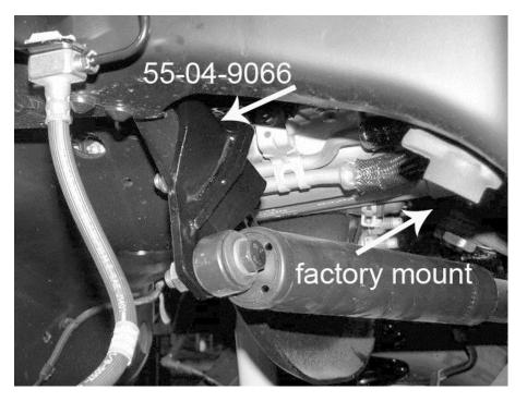
front axle via a bracket located in front of the coil spring's lower seat. Unplug the vacuum line where it passes through this bracket then unbolt the bracket from the axle.
