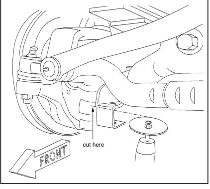
should be positioned between the stud and the axle bracket. Tighten (64).
