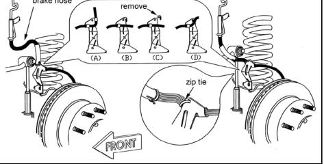
and hub vacuum lines as necessary to gain an adequate amount of slack with the suspension at full extension.
