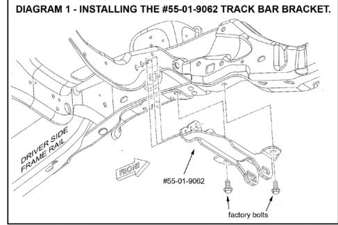
track bar bracket attaches. Often there is an excessive amount of undercoating build-up on the crossmember, especially on the back (rearward facing) portion of the crossmember where the undercoating has pooled up. Scrape off any excessive undercoating to prevent the track bar bracket from loosening over time.
