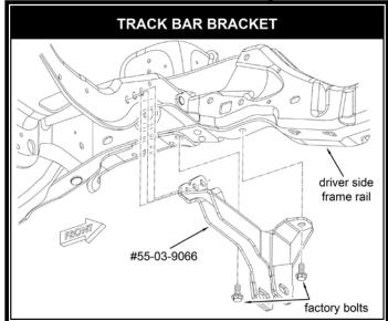
its mounting cup then unbolt the cup from the frame.
