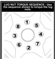
**WARNING:** Retighten lug nuts at 500 miles after any wheel change, or anytime the lug nuts are loosened. Failure to do so could cause wheels to come off while vehicle is in motion.
