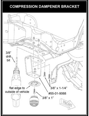
supplied 3/8" x 1-1/4" bolts, pointing up, as shown. Place the washers on the frame side, install nyloc nuts and tighten (23).
