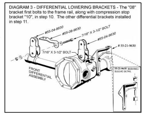
□ Loosely attach the remaining two "04" brackets to the frame. Use the factory bolts, pointing forward. Hand tighten only.
