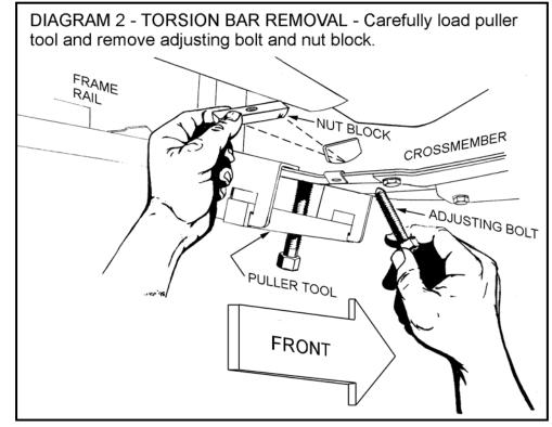
□□ [DIAGRAM 2] Load the bars using a torsion bar puller tool (discussed in the
