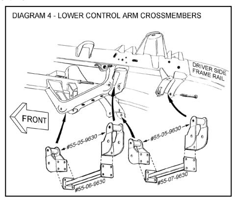
front and rear crossmember tubes. Use the 3/8" x 1" bolts / Nyloc nuts; again, hand tighten only.
