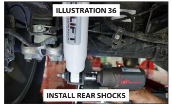
60. Install a new sleeve (24-5704) into each shock bushing.
