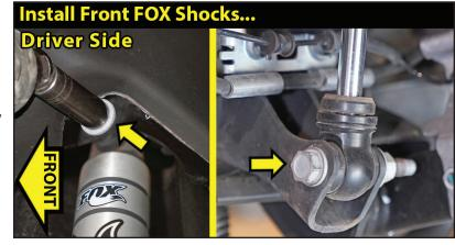
Snug tighten only. Shocks will be tightened completely when the vehicle is set on the ground.
