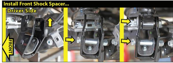
hole of the bracket/factory mount. Install 3/8" flange nut. [9/16 wrench / 9/16 socket]
