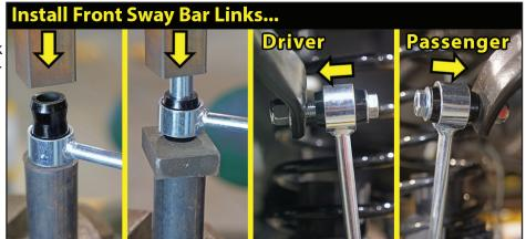
Snug tighten only. [19mm wrench / 19mm socket]
