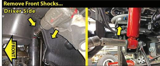
Remove shocks. Retain the shocks and shock mount hardware.
