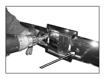
Bowtie is larger than OE bowtie Install mounting studs on bowtie Center bowtie on grille (mounting studs center close to OE holes but will not fit) Mark the area needed for mounting holes Use a drill bit to enlarge / drill holes in bowtie area (see arrow in picture) Center bowtie onto grille shell (slide studs into mounting holes) Install washers and nuts from behind shell
