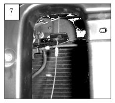
Make a loop (large enough for your index finger) with the cable provided (6); use an eyelet to crimp the loop. Feed the other end of the cable through the hole on top of the grille; then through the hood release (4 & 7).
