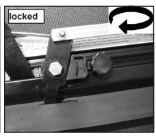
The Deuce cover can be locked while the cover is rolled up or in the open position as shown above.
