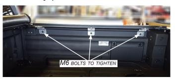
**STEP 5:** To assure adequate water sealing of the Pro X15 rails to the trucks bed rail caps, push the Pro X15 rails againts the truck box and with force still applied tighten the pan head screws.
