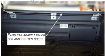
STEP 6: Tighten all fasteners. Repeat steps 1-5 on driver's side.
