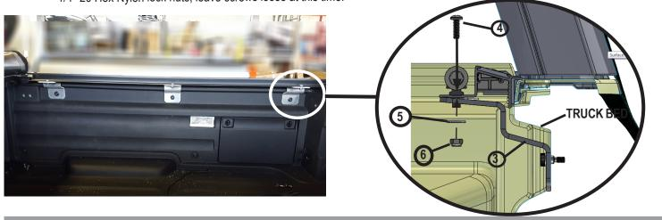
**STEP 4:** Tighten all six M6 shoulder bolts, make sure the brackets fit tight to the truck bed side. At this time the Pro X15 rails should be able to move in and out slightly.
