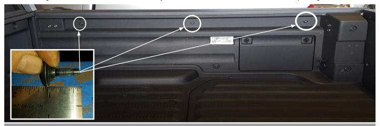
**STEP 2:** Mount brackets on driver and passenger side using the factory installed M6 Shoulder bolts. Leave finger tight for now.
