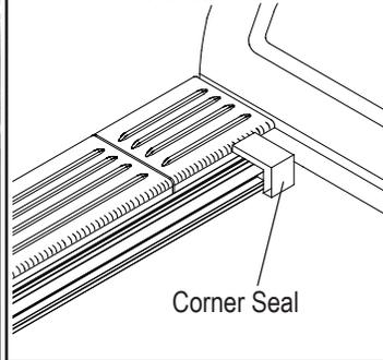
**STEP 5.** Apply weather seal across the front bulkhead, trimming ends to match bed cap contour.
