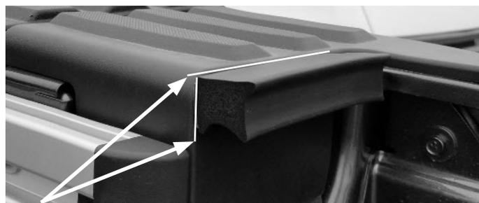
Align seal flush along the top edge of the bed cap and the inner edge as shown.
