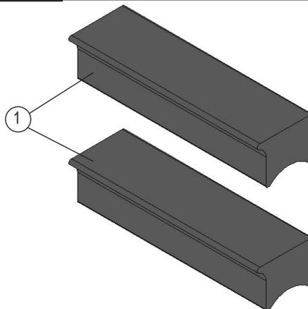
**STEP 2.** Once cover Rails are installed, clean the area shown below on Driver and Passenger side with wet rag.
