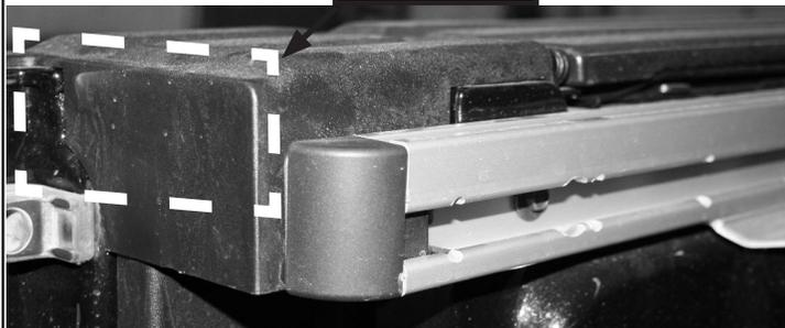
**STEP 3.** Apply Seal on Driver and Passenger Side as shown below.
