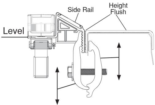
If side rail tilts up or down, Level the side rail tilt by adjusting clamps up or down as needed.
