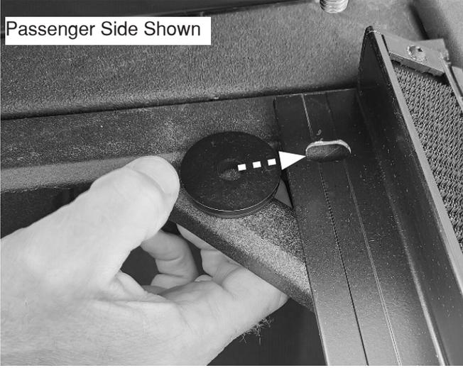
**4** Align the black washer's hole to the side rails oblong hole. Move the front header in place and align the screw in the header with the hole in the rail and washer. Drop the header down so the screw extends through the holes.
