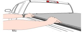
We recommend securing the hook and loop fastener along the entire length of both side rails before driving the vehicle. Simply pull the fabric over the hook.
