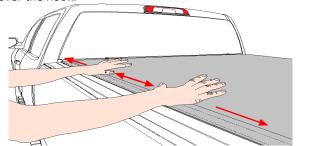
Next, run your hands down both sides of the cover. This will prevent wind from lifting the cover and causing possible damage.
