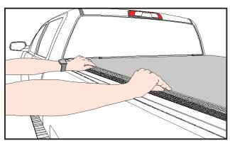
Engaging Hook and Loop, Step One: After rolling Engaging Hook and Loop, Step Two: With the cover the cover closed, grab the fabric loop flap and evenly pull loop over the hook track engaging the loop to the hook track. Avoid pulling fabric flap straight up.
