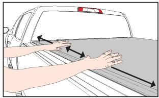
closed and both hook and loop engaged, use the palms of your hand to firmly push the loop strip into the hook track. Do this to both driver and passenger side up and down the entire length of the loop seams.
