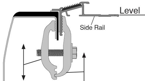
If side rail tilts up or down, Level the side rail tilt by adjusting clamps up or down as needed.
