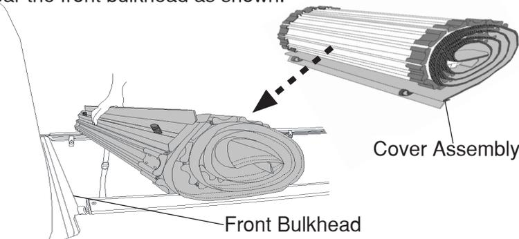
Rotate the front header over and align the screws with the holes in the side rails.
