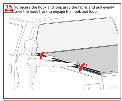
Once the side of the hook and loop are engaged, use the palm of your hand to firmly push the loop strip into the hook trackthe entire length of the cover. This will prevent wind from lifting the cover and causing possible damage. Do this on both driver and passenger sides.
