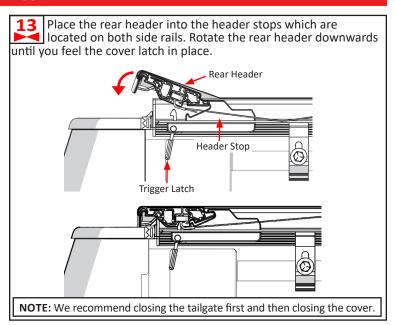
A clicking sound will indicate a correctly installed cover. Next secure the hook and loop fastener along the entire length of both side rails before driving the vehicle, see steps 15 and 16.
