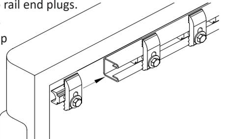
**4** Position clamp here Position Rear tie down here Position Front tie down here Position clamp here
