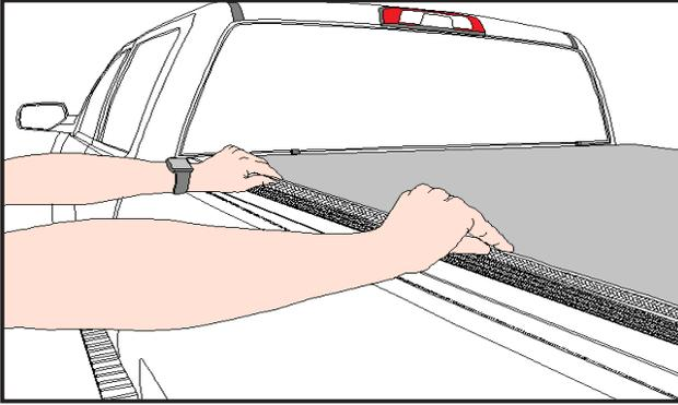
**Engaging Hook and Loop, Step One:** After rolling the cover closed, grab the fabric loop flap and evenly pull loop over the hook track engaging the loop to the hook track. **Avoid pulling fabric flap straight up.**
