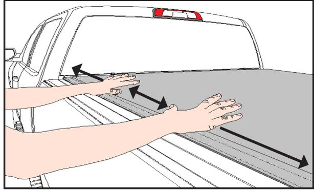
**Engaging Hook and Loop, Step Two:** With the cover closed and both hook and loop engaged, use the palms of your hand to firmly push the loop strip into the hook track. Do this to both driver and passenger side up and down the entire length of the loop seams.
