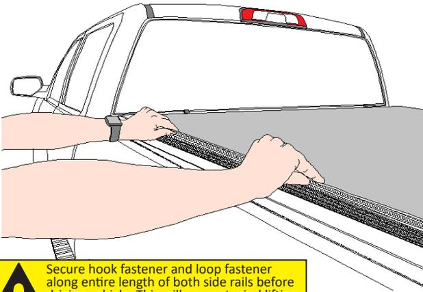
**!** Secure hook fastener and loop fastener along entire length of both side rails before driving vehicle. This will prevent wind lifting the cover and causing damage.
