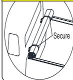
Before driving with cover open, **BOTH STRAPS MUST BE SECURED TO RETAINING LOOPS.** Failure to do so could cause accidental release of the cover, resulting in personal injury or property damage.
