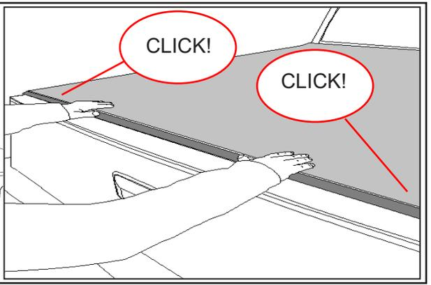
**19** PREFERRED METHOD OF CLOSURE: Close tailgate, then close cover on top of tailgate. This method will not work with some truck applications. Use alternate method instead.
