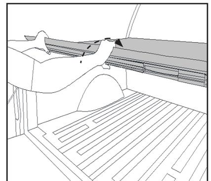
**23** To drive with the cover in the open position, secure the cover by placing both retainer hooks into the retainer loops. **You are ready to drive with the cover in the open position.**
