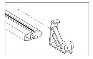
2. Tighten the twist knob until the Load Stops do not move and are locked in place.
