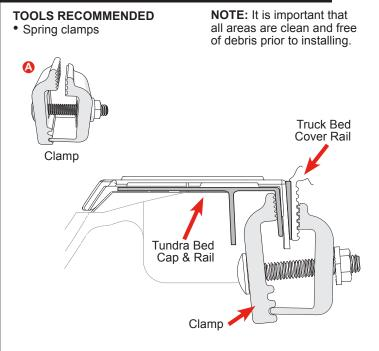
Position the driver side rail against the truck's bed rail. Begin clamping the driver side rail to the truck bed. Start in the middle and evenly space 3 clamps (A) along the rail. You should leave approximately 8" on each end of the rail. Finger tighten the clamps, making sure the teeth properly engage with the grooves of the side rail. Repeat on the passenger side rail.
