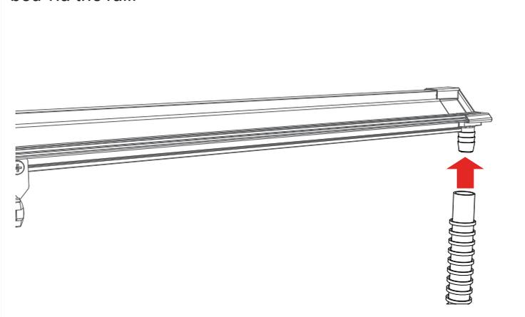
**11** Depending on year of your truck - use a 5/8" drill bit to make the existing hole bigger in a newer truck through the floor on driver and passenger side or through the plugs on an older truck, then run the end of the drain tubes through that 5/8" hole on both sides.
