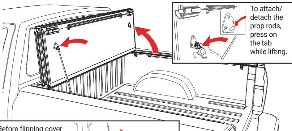
To attach/detach the prop rods, press on the tab while lifting.
