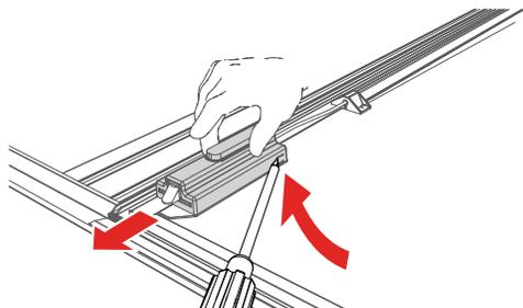
Use a screwdriver to partially pry open the tab on the latch housing. At the same time slide the housing away from the latch assembly.
