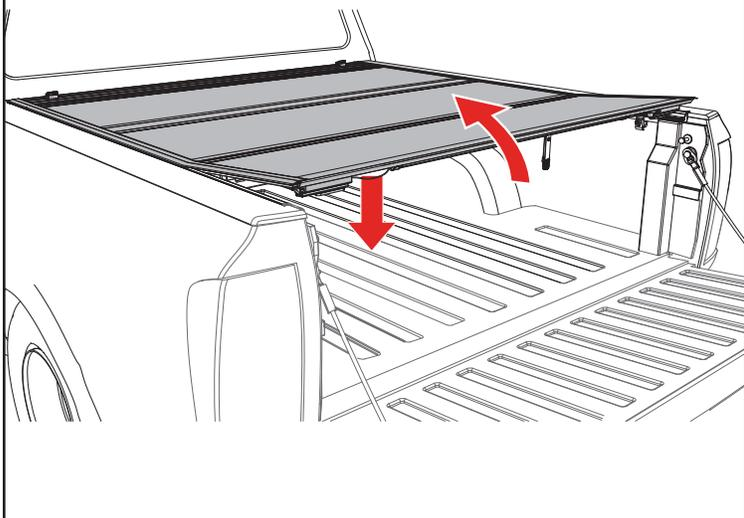
**FOLDED UP POSITION:** To drive with the cover (C) in the folded up position, use the straps and buckles provided with the cover. Attach the buckle at the bulkhead, then pull the strap to take up the slack and secure the cover.
