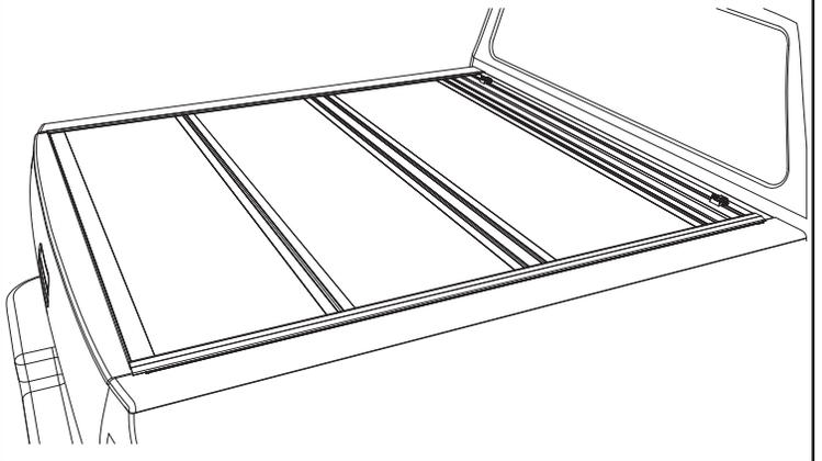
**OPENING COVER:** Lower the tailgate and pull the cable on either side. While pulling on the cable lift the panel up and towards the cab.
