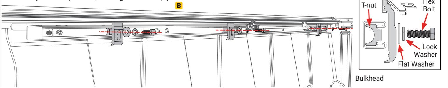
**9** Align the driver side rail (B) with the drain tube fitting going towards the cab of the truck and pushed up against the bulkhead. Position one clamp assembly 6-8 inches from the bulkhead, one clamp assembly in the middle and one clamp assembly as close to the tailgate as possible. The clamps should be evenly spaced along the rail. Tighten the bolts to 10 ft/lbs of torque with a 1/2" wrench or socket. **CAUTION: Do NOT overtighten.** Repeat on passenger side rail (C).
