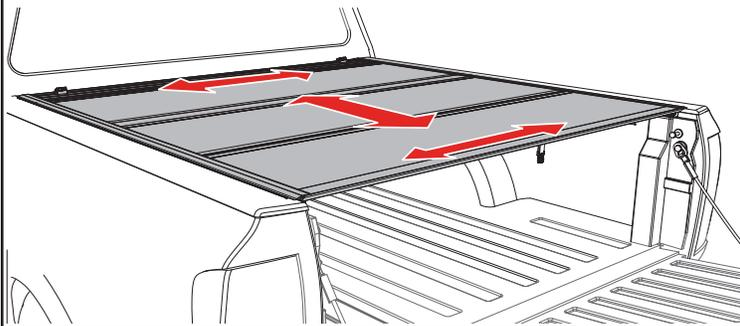
**17** The rear edge of the cover (A) and tailgate seal should rest on top of the tailgate. **You are ready to drive with your cover in the closed position.**
