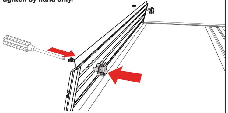
**14** Set the cover (A) in the folded position on the side rails (B & C) towards the cab of the truck. Confirm the cover is evenly spaced between the rails.
