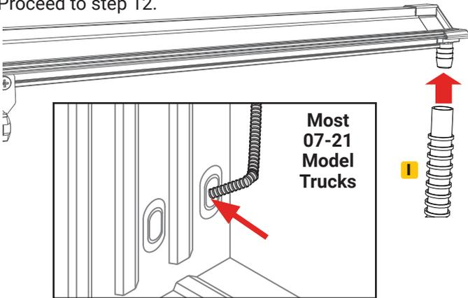
**4 For Trucks With Cargo Management System:** Remove the factory end caps from both ends of the bulkhead utility rail.
