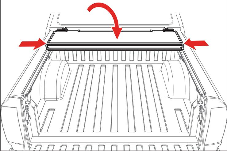
**15** Confirm the retainer clamps (F) are positioned around the side rails (B & C) correctly as shown below. Tighten the retainer clamps by turning them clockwise until the lock washer is secure.
