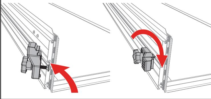
**13** Position the buckle ends (H) with the open side facing the bed cover panel. Use a screwdriver to install the two buckles into the pre-drilled holes on the front header panel with the provided screws (I). **DO NOT use a screw gun, securely tighten by hand only.**
