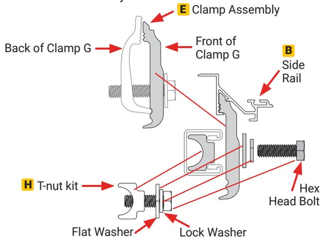
**6 Installing T-nut Kits in Cargo Management System:** Remove the factory end cap from tailgate end of the accessory rail. Insert three T-nut kits (H) into the end of the accessory rail and put the end cap back in. Repeat on passenger side.
