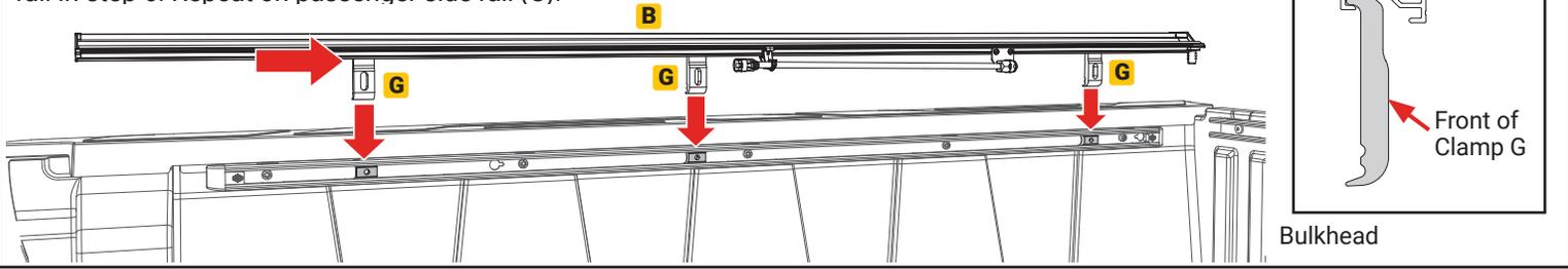
**8** Place the driver side rail (B) on to the truck bed rail. Use the 5/16" hex head bolt, 5/16" flat washer and 5/16" lock washer from T-nut kit (H) when installing driver side rail (B) to truck bed with accessory rails. Repeat on passenger side rail (C).
