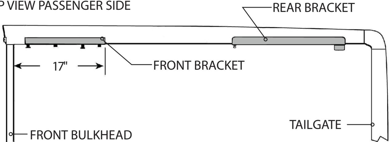
Adjust the lock strikes up or down accordingly. With the tailgate down adjust the lock strike to allow approximately 1/8" (3mm) play in the cover up and down.
