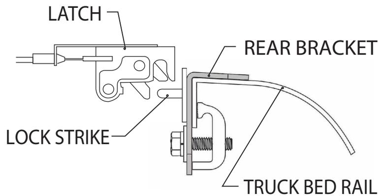
It may be necessary to adjust the latch side to side, to do so loosen the two latch mounting bolts, adjust latch and tighten.
