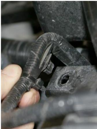
3. Undo two MAF sensor wire retaining clips.
