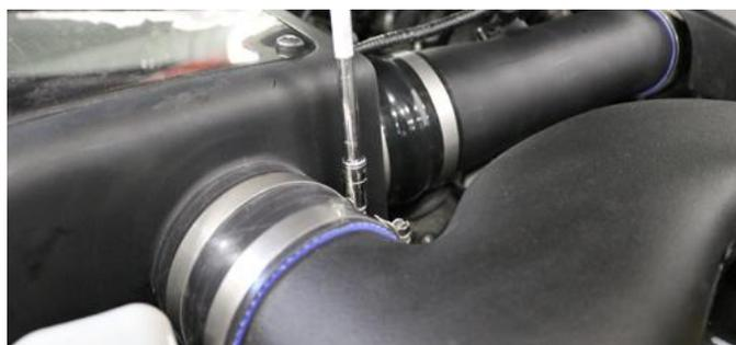
**16.** Tighten clamps using an 8mm socket.
