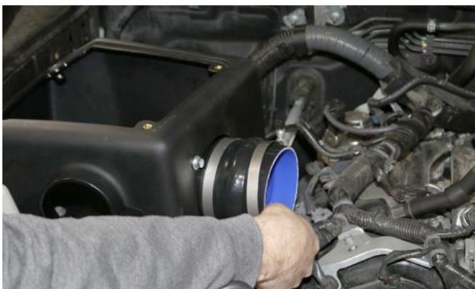
5. Insert two #64 clamps on hump hose, and place hump hose on filter adaptor.
