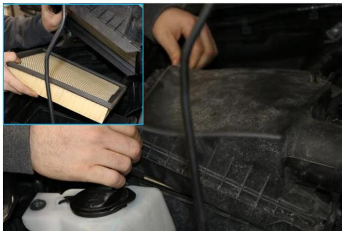
7. Unclip the factory lid and remove. Remove factory filter from factory air box.
