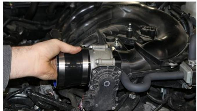
4. Insert two #56 clamps on reducer, and place small end of the reducer on the throttle body.
