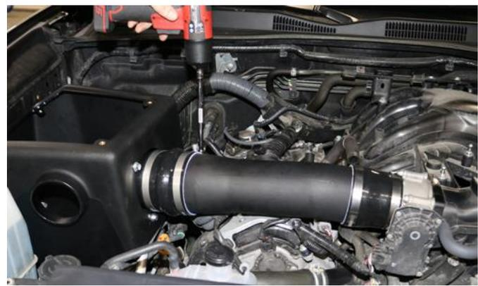
6. Insert the large end of the duct into the hump hose and the other into the reducer. Adjust as needed. Tighten all clamps using a ratchet and 8mm socket or flat head screwdriver.
