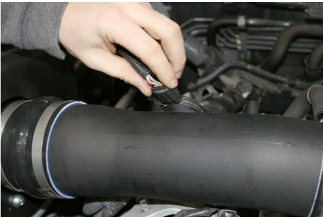
9. Re-attach MAF sensor wire.
