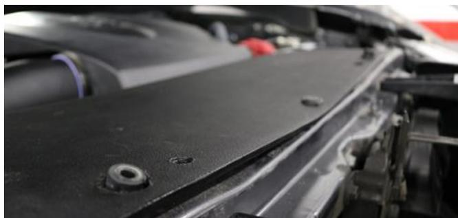
**15.** Use clip from **Install Step 12** to secure scoop.
