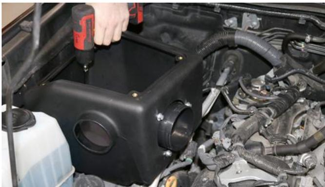
3. Insert Volant air box into vehicle and mount using two of the bolts from **Removal Step 8** of removal. Use a ratchet and 12mm socket to mount box to factory location.
