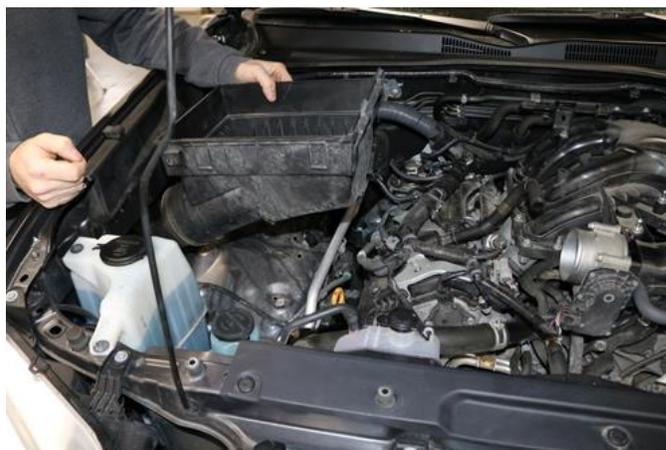
9. Using a Philips head screwdriver, remove MAF sensor from stock lid.
