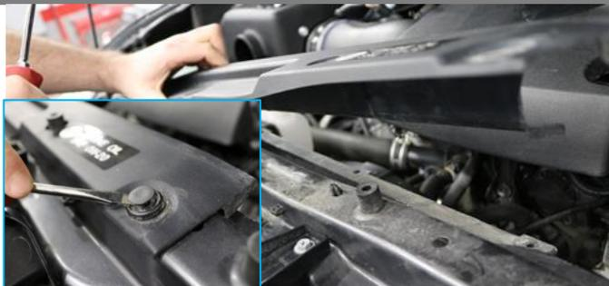
**12.** Remove 7 retaining clips using pry tool. Save 1 clip for **Install Step 15**. Remove tray cover.
