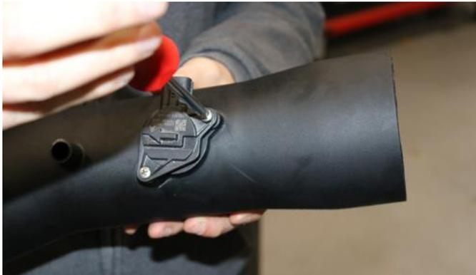
1. Install MAF sensor into Volant air duct using provided MAF Screws and screwdriver. Place rubber washers between MAF sensor and duct.
