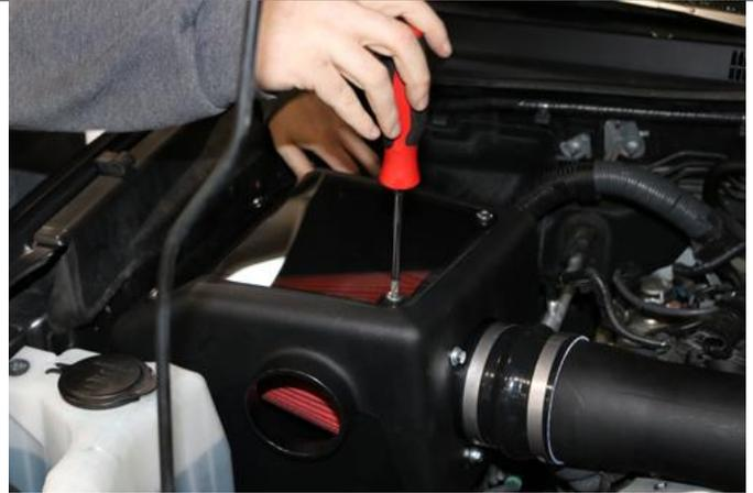
8. Install Volant lid onto air box, secure with provided four truss head screws with rubber washers using a Philips head screwdriver.
