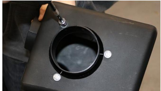
2. Install filter adaptor onto Volant air box with provided hardware using a ratchet and 10mm socket.
