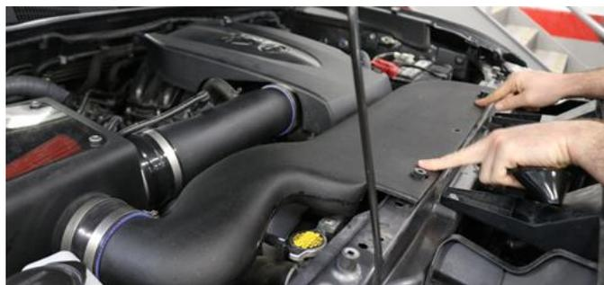
**14.** Attach straight sleeve onto air box and slide scoop into place over hood rubber stops.
