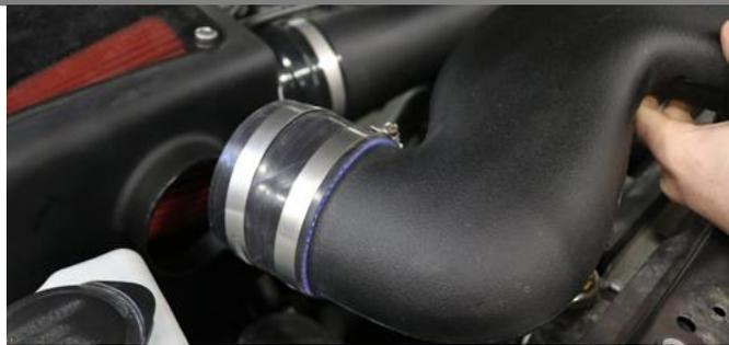
**13.** Place two #56 clamps and straight sleeve onto the Volant RAM Air Scoop.
