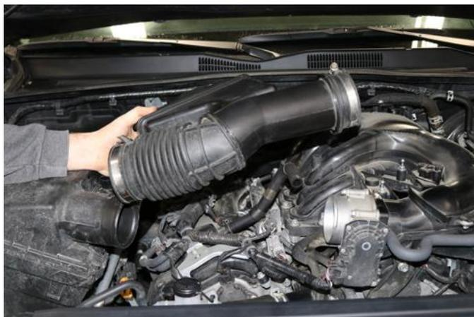
6. Remove factory air duct.
