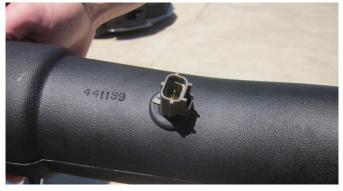
9. Install air temp sensor from Removal Step 9 with the tab facing the closer end of the duct.
