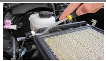
**5.** Remove the two plastic wire retention clips from back of factory air box
