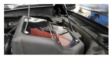
**16.** Install lid using provided 4 truss head screws with rubber washers and Philips head screwdriver.
