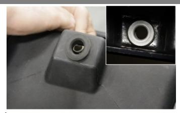
1. Insert the factory grommet from Removal Step 7, then install the metal bushing into grommet from inside box as shown.
