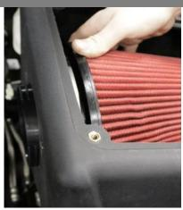
7. Insert the filter into the air box with the adapter side down. Rotate the top of the filter down into the air box and rotate the filter around and push the adapter through air box.
