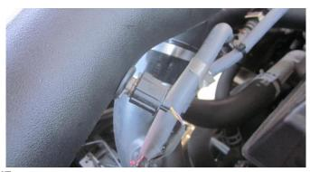
**15.** Clip wiring harness on air temperature sensor.
