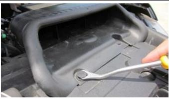
**6.** Remove the two plastic clips from the factory air scoop. Save clips for **Install Step 5**.
