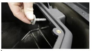
**4.** Attach the Volant air box to the fender with the bolt from **Removal Step 4** using a ratchet and 13mm socket.
