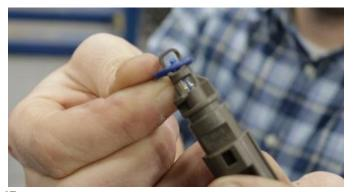
**10.** Remove O-ring from the temp sensor.
