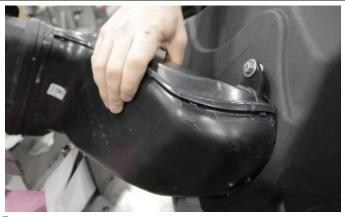
Install factory scoop to Volant air box using provided 6mm-25 bolt with flat washers, lock washer, spacer, and nut using 10mm socket or wrench..
