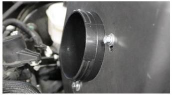
**8.** Attach the filter adapter to the Volant air box using the provided 3 bolts, flat washers, and lock washers and a 10MM wrench or socket.
