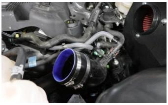
11. Install the straight sleeve onto lower factory inlet with #64 clamp. Tighten clamp using a ratchet and 8mm socket or flat head screwdriver. Leave clamp on open end of straight sleeve loose.
