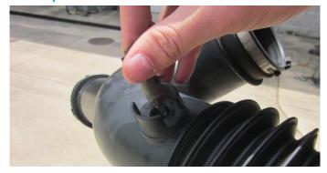
**9.** Remove the air temp sensor from factory duct. Save for Install Step 9.
