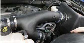
**14.** Adjust air duct as necessary and tighten all clamps using a ratchet and 8mm socket or flat head screw driver. **NOTE:** Make sure to tighten the filter clamp as well.
