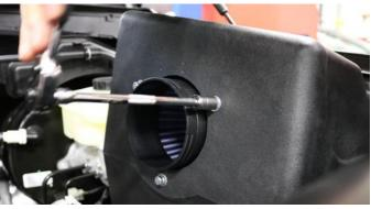
7. Secure the filter adapter to the Volant air box using a 10mm socket and three M6-16mm bolts, lock washers, and flat washers.
