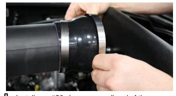
**9.** Install one #56 clamp on small end of the reducer, and one #64 clamp on larger end of reducer. Place small end of reducer onto straight end of Volant air duct.
