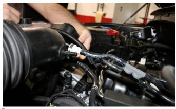
**3.** Disconnect both vent connections from the rear of the factory duct.
