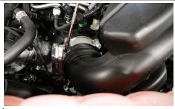
Loosen the throttle body clamp using a 7mm socket.
