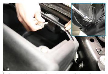
4. Use the bolt saved from Removal Step 7 to attach the Volant air box to the fender with a 13mm socket.
