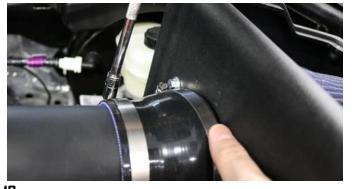
10. Insert the air duct onto the straight sleeve on the throttle body and large end of reducer onto the filter adapter. Adjust Volant air duct to proper fit and tighten all clamps using an 8mm socket or flat head screwdriver. NOTE: Also tighten the filter's clamp at this time.
