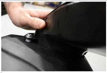
2. Attach the factory air scoop onto the Volant air box using a 10mm and socket and wrench. Using the provided hardware; place the .625" flat washer on the M6-25mm bolt through the factory mounting location of scoop. Place the provided .25" spacer between the scoop and Volant air box. On the inside of the air box place the .75" flat washer on bolt, followed by lock washer and M6 nut.
