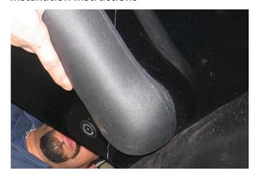
8. Insert the 3" opening of the Volant Riser Duct into the hole on the fender and into the sleeve. Clamp both ends of the sleeve with two #48 clamps using a 5/16" nut driver. With the ¼" washer, lock washer and nut bolt the set screw to the vehicle from the inside of the fender and tighten with a 7/16" open wrench. Note: This will need two people.
