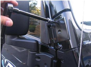
Bolt the Volant Snorkel Bracket onto the windshield bracket using the stock counter sink bolts.
