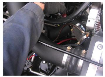
12. Clamp both ends of the 3" sleeve with two of the four #48 clamps to hold the Volant Down Pipe to the bottom of the filter box.
