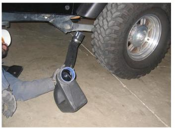
11. Attach the short snorkel onto the filter box by running it from underneath the vehicle and work your way up to the filter box and align the sleeve to the 3" hole on the fender.
