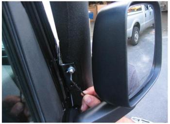
5. Mount the Volant Riser Duct to the Snorkel Bracket using the two ¼"-20 Socket Button Screws and tighten with a 5/32" Allen key.
