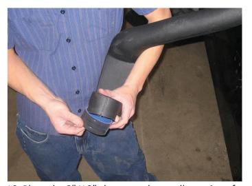
10. Place the 3" X 3" sleeve on the small opening of the Volant Down Pipe and the 3 ¼" X 2" sleeve on the other end of the short snorkel.
