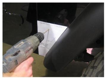
6. Once the template is lined up and taped to the fender, drill two 1/8" pilot holes as noted on the template.
