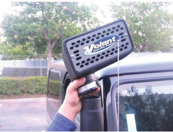
13. Once the Volant Snorkel is mounted and bolted on the vehicle place the Volant Scoop Top to the top of the Volant Riser Duct and clamp it down with a 5/16" nut driver
