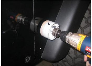
7. Remove the template from the fender. Drill a 3" hole with a hole saw on the top 1/8" pilot hole and a 3/8" hole with a drill bit on the lower pilot hole.
