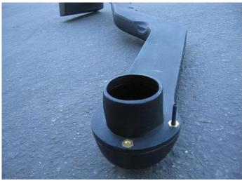
9. Screw the ¼" -20 set screw using a 1/8" Allen key to the molded insert on the right side of the opening of the Volant Riser Duct.
