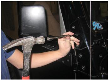
Remove the two top counter sink bolts from the front windshield bracket with a torx key #40 Note: In order to loosen the bolts, tap them lightly with a hammer to loosen the Loc tite.
