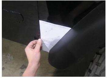
4. Align template along the side base of the jeeps passenger fender. Tape the template to the fender.
