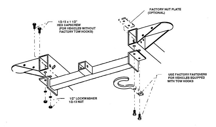
3. Install the multi--mount receiver to the vehicle frame, as shown above. Use the supplied fasteners if the vehicle was not equipped with factory tow hooks. If the vehicle has factory tow hooks, they can be re-installed using the factory fasteners and nut plate, (REFER TO FIGURE 1). Torque all fasteners to 40-ft/lbs.
