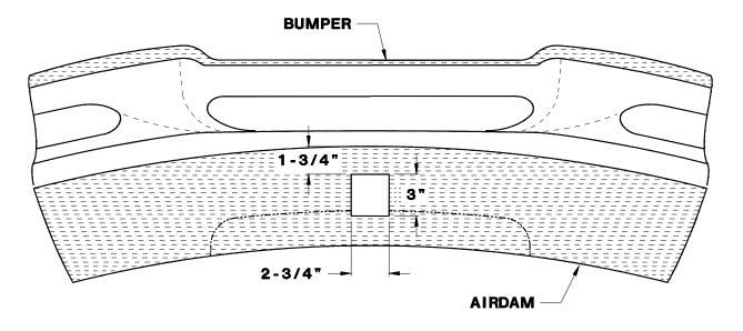
Cut Airdam as shown above for **Front Receiver**.
