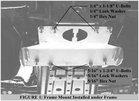
of the frame as shown in Figure 1. Four
