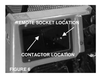
2. Refer the WINCH OPERATOR'S MANUAL for remote socket installation. See Figure 6 for recommended socket location.
