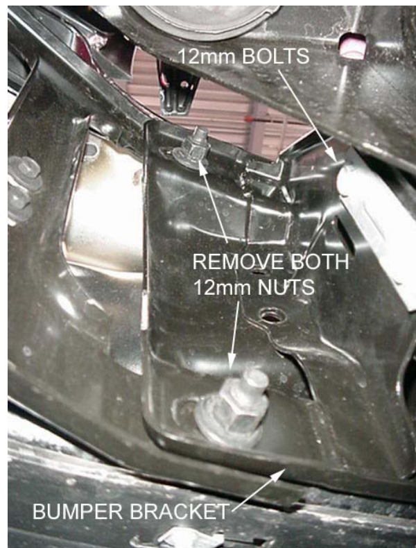
Figure 2 Bumper retaining nuts, (outboard left side shown)
