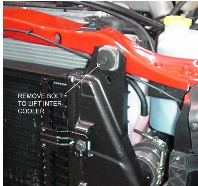
Figure 3 Intercooler retaining bolt (diesel only, left side shown)
