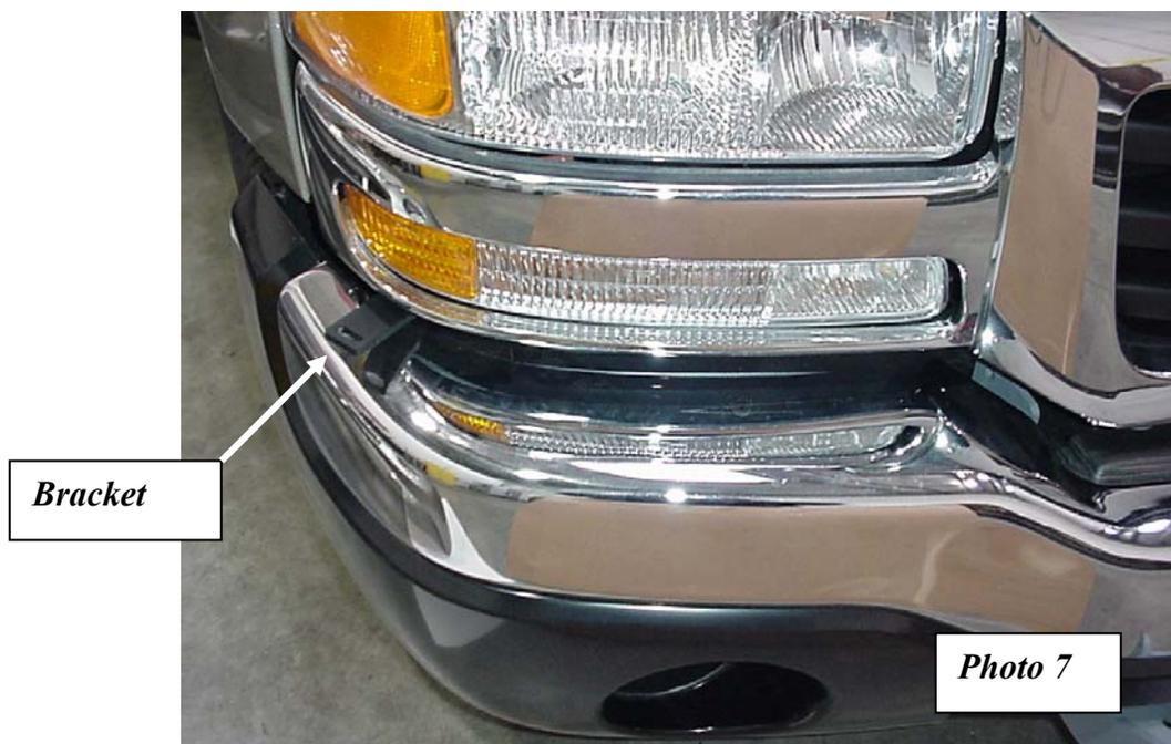
7. Align the slot in the bracket with the hole in the bottom of the Brush Guard. Install the 1/4" self-tapping bolt from the bottom up and tighten securely. **Photo 8**. Tighten the 3/8" bolt at the Bracket to bumper connection.
