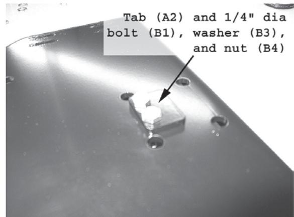
Figure 1 Attach Tab to Plow Mount
