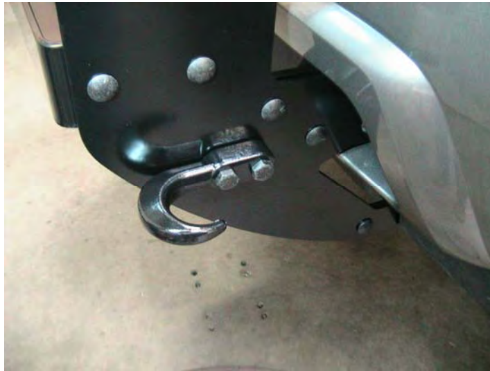
Figure 8 Installing Tow Hooks
