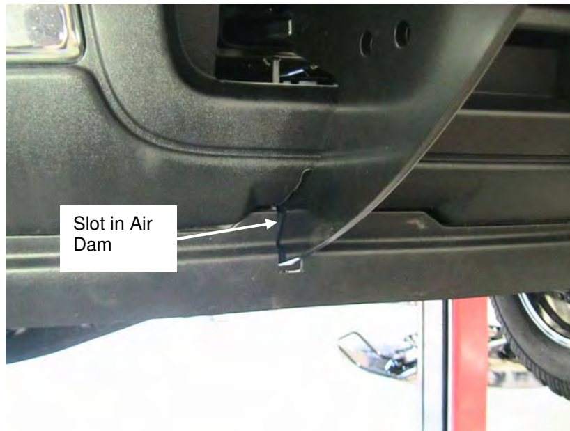
Figure 6. Side Member Through Slot. (GMC Sierra)
