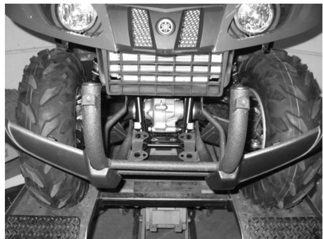
Figure 6: Rotate grab bar forward
