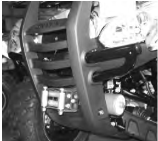
Figure 21 Front Fascia Reinstalled
