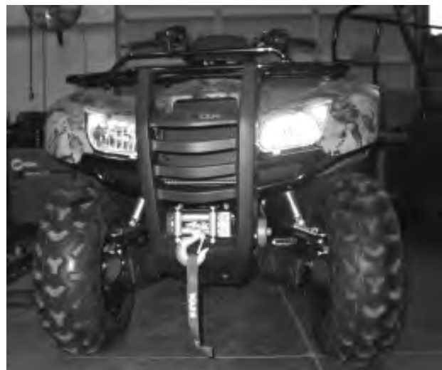
Figure 24 Winch and Mount Installed
