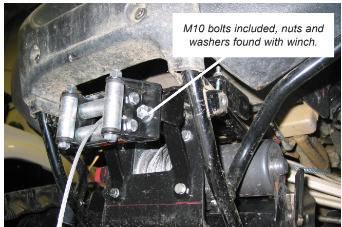
Figure 7 Attach Roller Fairlead
